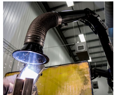
This powerful fume extractor can help protect two operators from fumes for heavy-loading applications.
