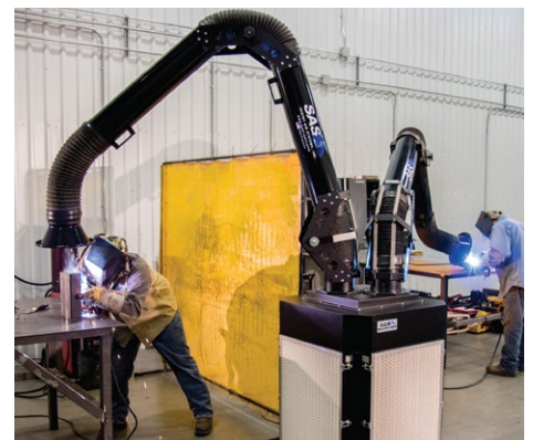
This powerful fume extractor can help protect two operators from fumes for heavy-loading applications.
