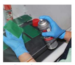
Close-up of operator spraying conformal coating under the 30" DSH.
